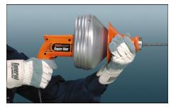
Gently squeeze the trigger and move the machine toward the drain opening. **DO NOT FORCE THE CABLE.** The job won't go any faster and you could kink the cable.
