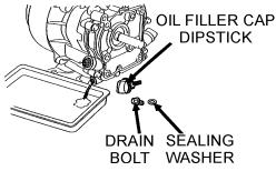
Figure 21. Engine Oil (Draining)
