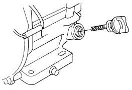
Figure 4. Engine Oil Dipstick (Removal)
