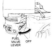
Figure 18. Fuel Valve Lever (OFF)
