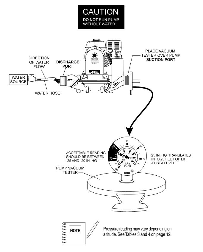
Figure 19. Pump Vacuum Tester
