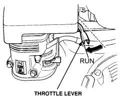
Figure 15. Throttle Lever (Run)
