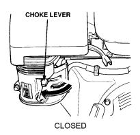
Figure 11. Engine Choke Lever (Closed)
