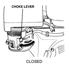
Figure 14. Choke Lever (Closed)
