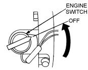
Figure 17. Engine ON/OFF Switch (OFF)
