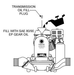
Figure 6. Transmission Oil Level
