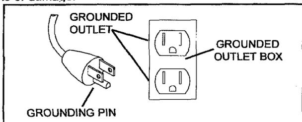
**▲ DANGER:** Improper installation of the grounding plug can result in electrical shock. If repair or replacement of the cord or plug is required, do not connect the grounding wire to either flat blade terminal. The wire with the green (with or without yellow stripes) insulation is the grounding wire and must be connected to the grounding pin.
