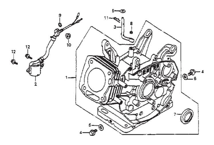
CYLINDER BARREL ASSY. (ELECTRIC START)
