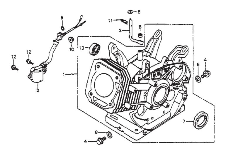
CYLINDER BARREL ASSY. (RECOIL STARTER)
