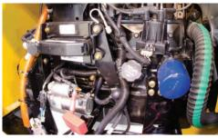
**ELECTRONIC FUEL INJECTION** (EFI) ENGINE. An 89 hp (66 kW) EFI GM engine performs well during cold-weather starts, provides improved fuel economy over comparable carbureted gas engines and increased/faster engine response under load.
