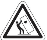
Raising an inflated tire more than 2" (5cm) above the ground or attempting to lift more than one wheel at a time may result in tip over, unexpected movement and serious injury or death. Always raise an inflated tire less than 2" (5cm) and only one tire at a time.
