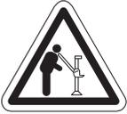
Unexpected movement of the jack handle may result in the user being struck causing serious injury or death. Always keep your head away from and out of the jack handle path of movement.
