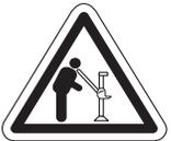
Using the jack on curved or tubular vehicle bumpers will result in the vehicle slipping off the jack and falling, causing serious injury or death. Use the Bumper Lift or Lift-Mate to lift most vehicles with curved bumpers or plastic bumpers.
