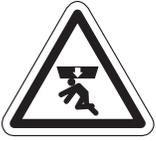
DO NOT USE THE JACK TO SUPPORT OR STABILIZE A LOAD. Using the jack to support or stabilize a load may result in unexpected movement and result in serious injury, being crushed and death. Always securely chock and block (stabilize) the load to be lifted. Never place any part of the body under a raised load without properly chocking and supporting the load.
