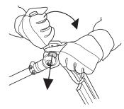
4 Fold down the cutting unit against the shaft.
