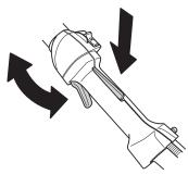
See instructions under the heading Start. Start the hedge trimmer and apply full throttle. Release the throttle trigger and check that the blades stop and remain stationary. If the blades move when the throttle trigger is in the idle position then the carburettor idle setting must be adjusted. See instructions under the heading Maintenance.
