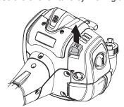
Remove the air filter cover and take out the filter. Wash it clean in warm, soapy water. Ensure that the filter is dry before refitting it.
