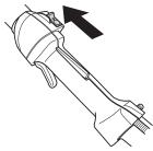
**CAUTION!** The stop switch automatically returns to the start position. In order to prevent unintentional starting, the spark plug cap must be removed from the spark plug when assembling, checking and/or performing maintenance.
