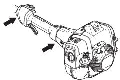
The machine's vibration damping system reduces the transfer of vibration between the engine unit/cutting equipment and the machine's handle unit.
