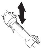
Check that the throttle trigger and throttle lockout move freely and that the return springs work properly.
