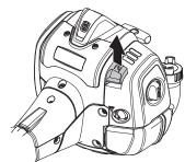
Hold the body of the machine on the ground using your left hand (CAUTION! Not with your foot!). Grip the starter handle, slowly pull out the cord with your right hand until you feel some resistance (the starter pawls grip), now quickly and powerfully pull the cord. **Never twist the starter cord around your hand.**
