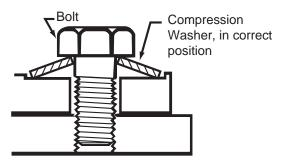
Fig. 5 - Proper installation of compression washer and bolts.
