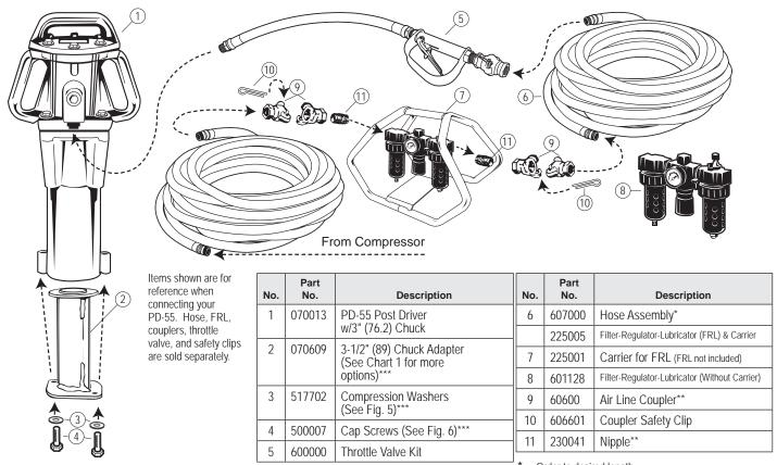
Fig. 3 - Connecting PD-55 to a post driving system.
