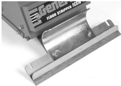
NOTE: Blade can be mounted offset for material removal under kick panels, cabinets and other inaccessible areas. Blade stiffener is included and must be used to minimize blade deflection. FIGURE 14
