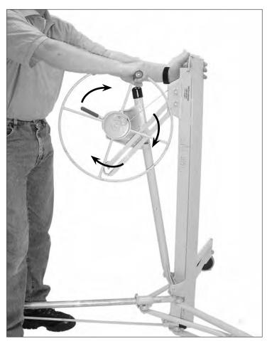
8. Hold the retaining hook in this position with your left hand and rotate the winch forward with your right hand. This will cause the winch assembly to fold up against the frame. When the slide bar contacts the frame, tighten the cable just sufficiently to hold the winch in the collapsed position.
