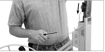
11. Pull the slack cable through the sheave pocket and slide the telescoping sections into the frame housing. As the telescoping sections lower into the frame, the slack cable will be drawn back up over the sheave.
