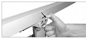
8. Mount the cradle on top of the telescoping section. Flip out the tilt latch to allow the cradle to tilt for loading and for hanging drywall on sidewalls and sloped ceilings.
