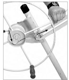
12. Feed the crimped end of the cable through the hole in the winch drum and secure it behind the mooring tab by hand pulling the cable snug as shown.
