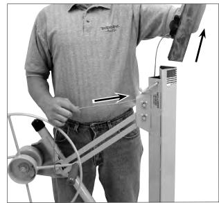
3. Remove the two telescoping sections completely from the frame housing. Pull the cable completely out from the frame along with them. Remove the "A" Section from the "B" Section as shown below. BE CAREFUL for loose strands or frays on the cable.
