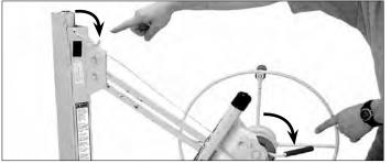
6. When the winch is fully extended, release the brake arm and swing the retaining hook away from the telescoping sections.
