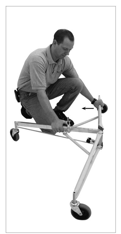
10. To collapse the tripod base, press down on the slide yoke pin clip and swing the legs in until they lock in the closed position.
