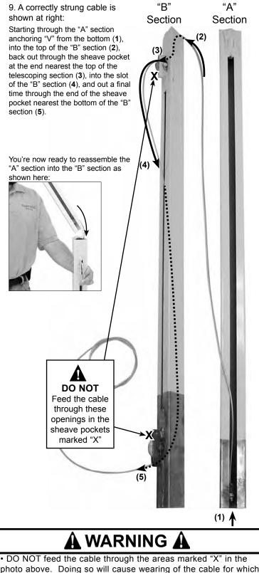
• DO NOT feed the cable through the areas marked "X" in the photo above. Doing so will cause wearing of the cable for which it was not designed which can result in failure of the cable. Failure of the cable while the lift is raised will result in a sudden and rapid lowering of the lift and load possibly resulting in serious property damage and/or serious bodily injury.
