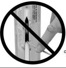
DO NOT feed the cable under the cable sheave on the frame as shown in this photo!
