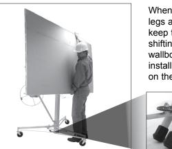
When the backstop legs are set, they keep the unit from shifting while loading wallboard or while installing the frame on the tripod base.
