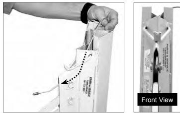
10. To reinstall the assembled telescoping sections, feed the crimped end of the cable through the frame sheave pocket from the top and over the top of the sheave as shown.
