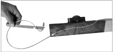
8a. Reload and insert the cable installation tool into the BOTTOM end of the "B" section as shown.
