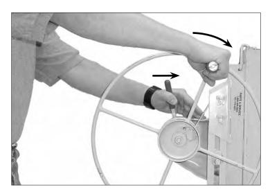
3. To move the winch into the working position rotate the winch forward slightly with your right hand while raising the brake arm with your left hand.
