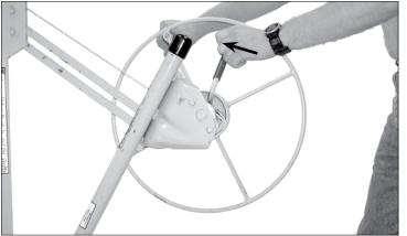
3. To lower the PANELLIFT<sup>®</sup> Drywall Lift control the backward rotation of the winch by grasping the winch handle with your right hand BEFORE releasing the brake with your left hand. ALWAYS use this two hand method when lowering the PANELLIFT<sup>®</sup> Drywall Lift. 4. The PANELLIFT<sup>®</sup> Drywall Lift will hold drywall in position on sidewalls and sloped ceilings in addition to level ceilings. The cradle also tilts up to 10<sup>°</sup> longitudinally.
