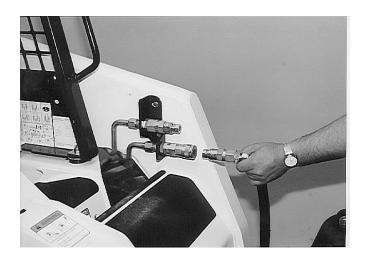
**NOTE:** Attachment is shipped with 12FJX (1-1/16" Female JIC Swivel) fittings on the ends of the lead hoses.
